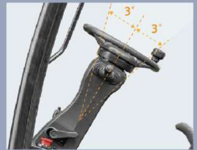
The angle of the hand wheel is adjustable
